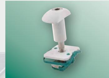
The innovative design of the BIS RapidStrut® Solar Panel Fixing allows a quick and reliable fixing of solar panels to Strut rail construction. The product is pre-assembled and delivered 'ready-to-use'. The plastic spring allows the assembly to be easily fixed into the rail. This innovative product is made from high-grade glass fibre reinforced plastic.
